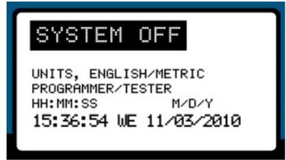
Figure 9-1 The clock shows the time in 24 hour format, the day of the week, in this example Wednesday and the date are shown in mm/dd/yyyy format.
