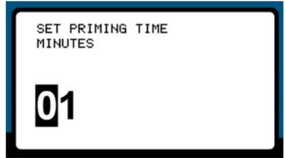
Figure 16-1 The Master Valve and decoder power will come on for the designated minutes before the first decoder in the automatic program is scheduled to turn on.
